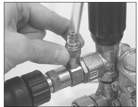
Figure 17 - Detergent injection adjustment
